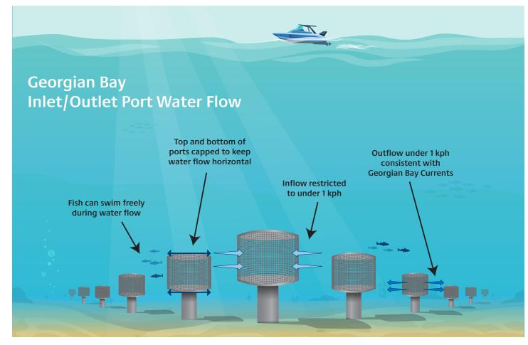
The 20 risers, spread out over 1.5kms in a semi-circle, will ensure water going into the system and being put back into deep water matches the currents found 800m off the shoreline of Georgian Bay.
